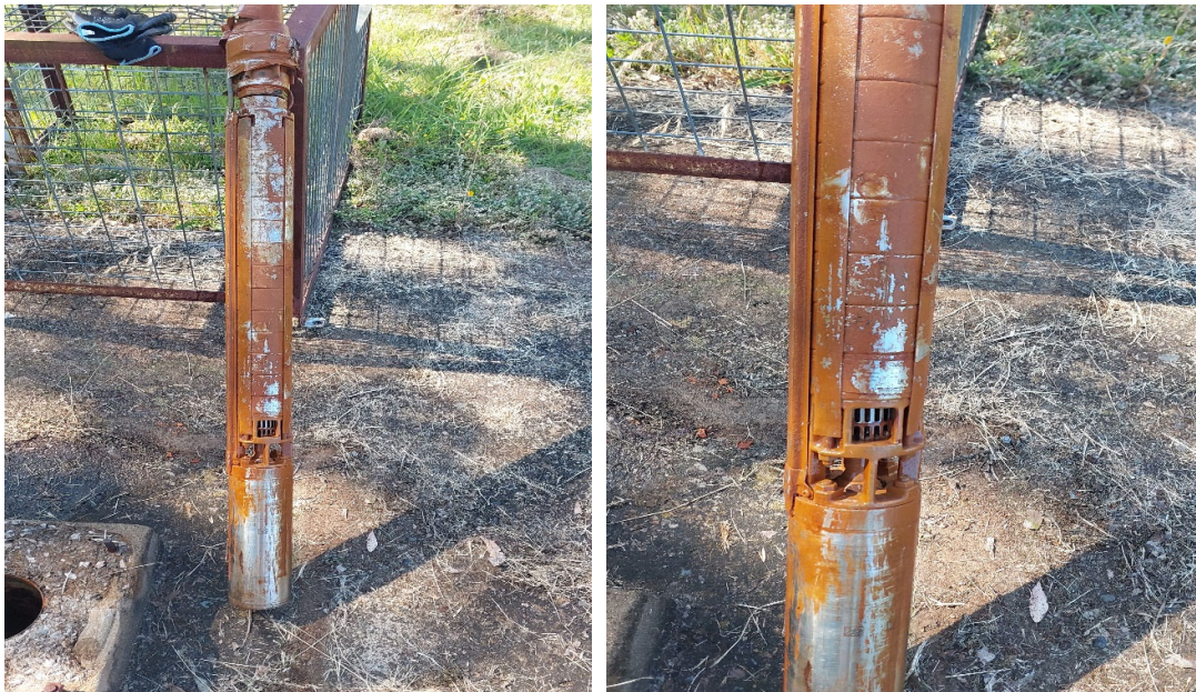
Condition of pumping equipment showing Iron Bacteria.
