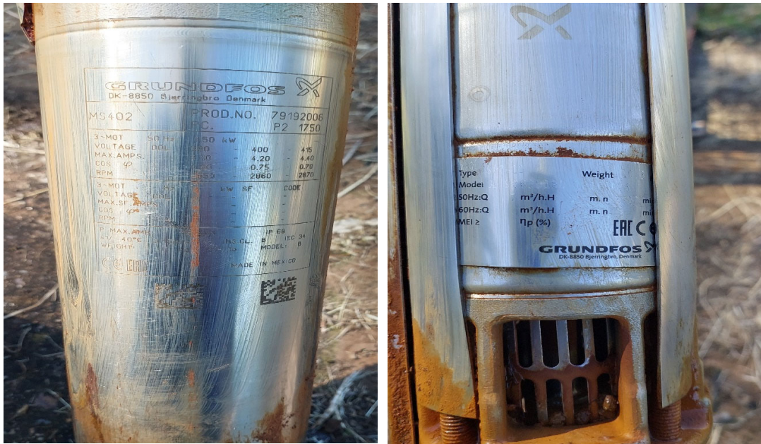
Identification plates as noted on submersible motor and wet end.
